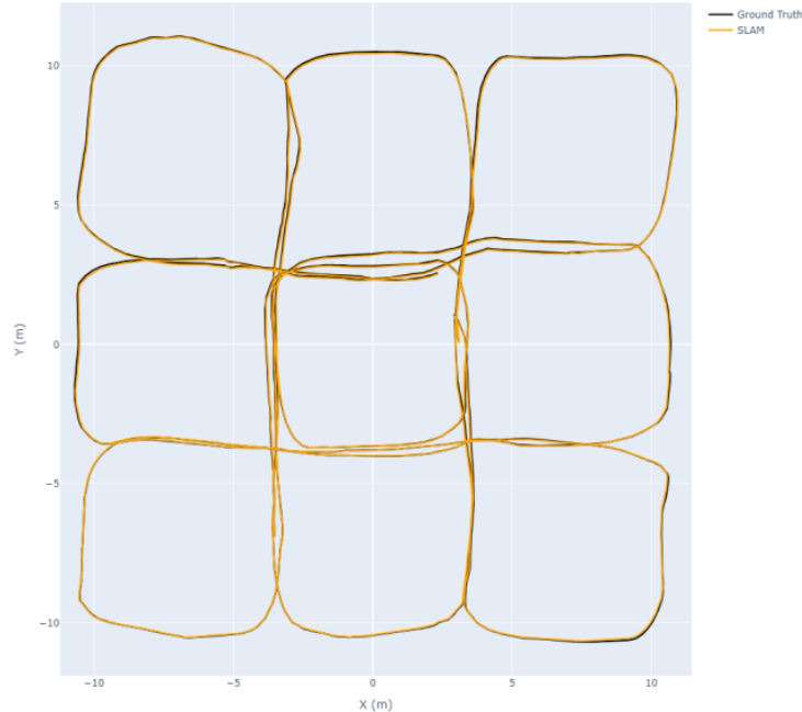
Figure 10: 2D trajectories from two different runs. In the right plot, multiple backup maneuvers were triggered as the planner disengaged from local obstacles. Despite this, our SLAM maintains low localization error through the entire trajectory.
