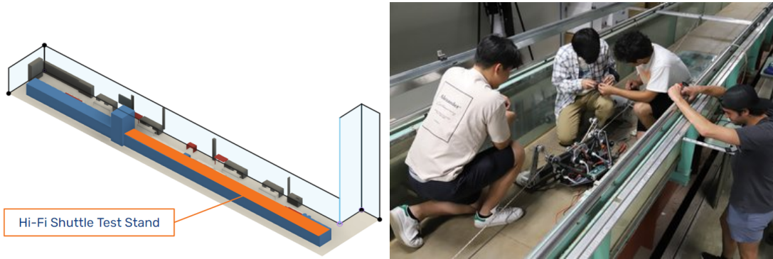
Fig. 16: Left: CAD of shuttle test stand in the lab. Right: Shuttle testing in the flume
