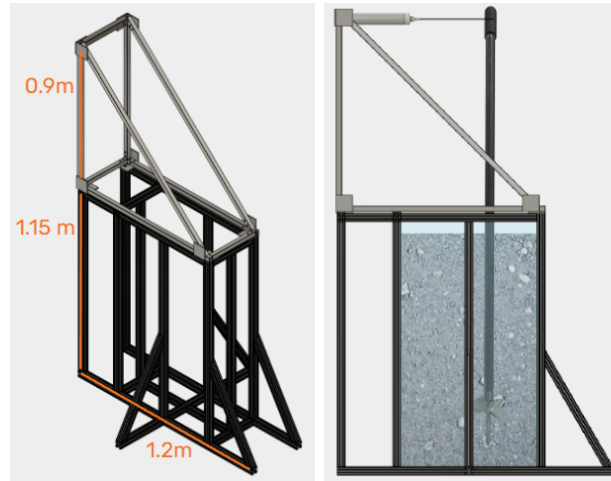
Fig. 17: CAD model of Stake Test Stand
