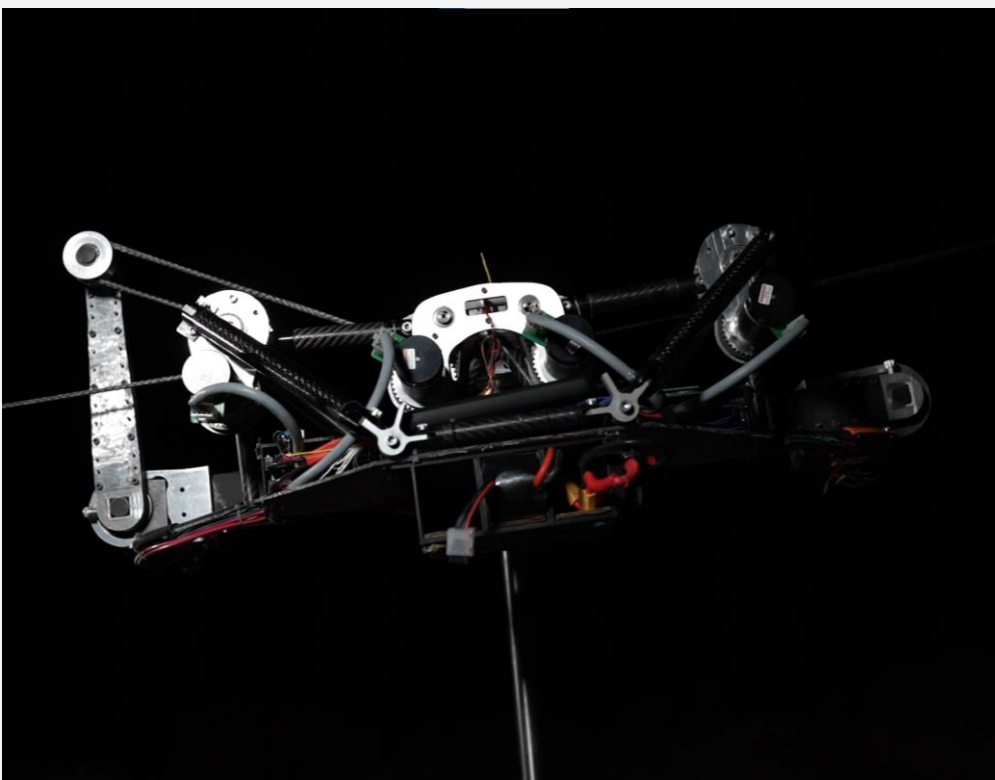
Shuttle performing stake transition and switching arms
