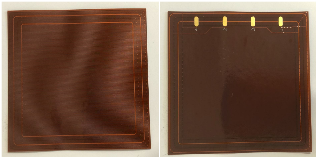
Fig. 33 Prototype of flexible PCB implementation of EDS board for durability. Despite the substrate being polyimide film, arcing was observed, and manufacturer delays and defects caused HOMES to remain with the rigid FR4-type PCB for later prototypes
