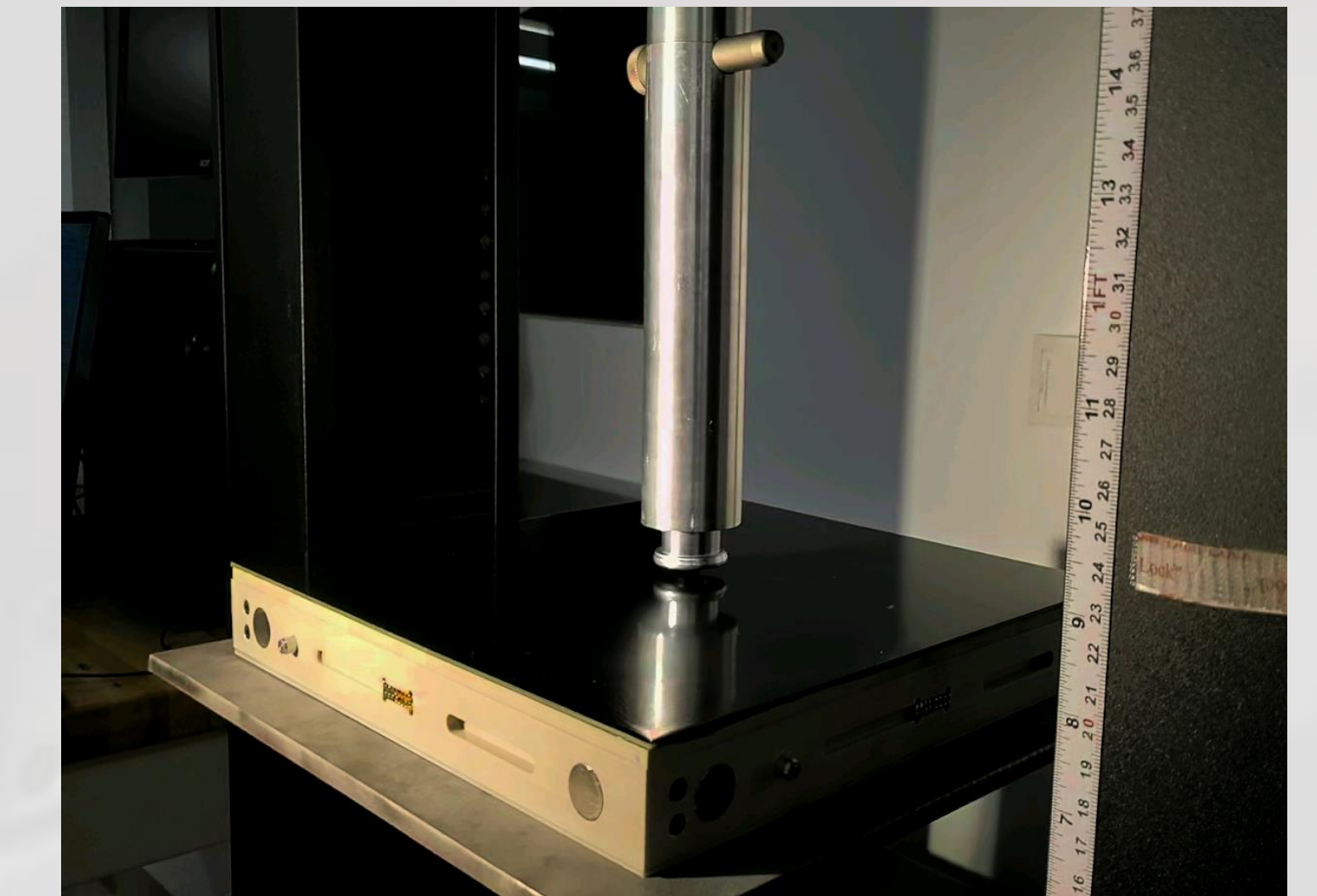
Quasi-static load test rig
